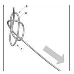
5 From the strings of the 3<sup>rd</sup> octave to those of the 0 octave, insert an anchor in the knot by using a 2-cm piece of gut string from the 5<sup>th</sup> octave; tighten by pulling the string in the direction indicated by the arrow, holding points B and C of the knot still
