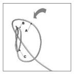
4 Tighten the loop on the knot in the direction indicated by the arrow, holding points B and C of the knot still
