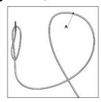
3 Overlap the loop on the knot in the direction indicated by the arrow, holding onto points B and C of the knot
